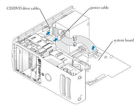
4 Slide the drive release mechanism to the right to release the shoulder screw and slide the drive out to remove it from the drive bay.
