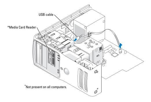
Disconnect the USB cable on the back of the Media Card Reader to the front panel USB connector on the system board (see page 71) and route the cable through the clip on the shroud.
