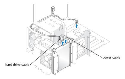
**2** Press in on the tabs on each side of the drive and slide the drive up and out.
